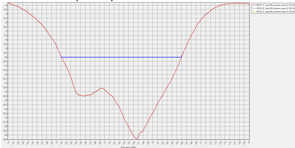
Figure 1 Antenna Matching (S11) vs Frequency, GHz, Measurements
