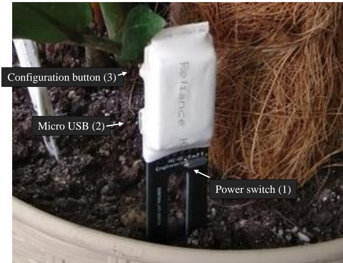
Figure 1 - Designation of sensor components (Sensor without enclosure)
